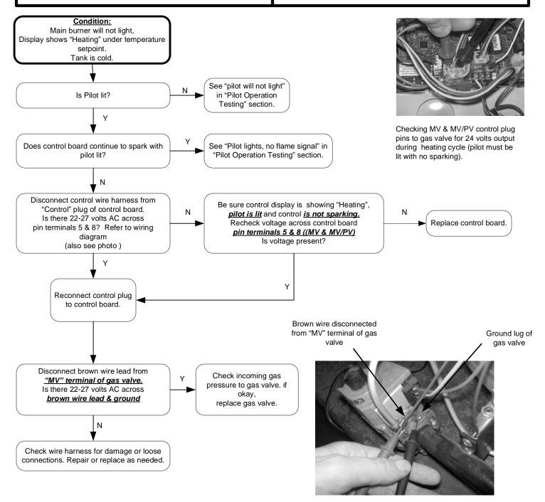
Checking main valve (MV) voltage to gas valve.
